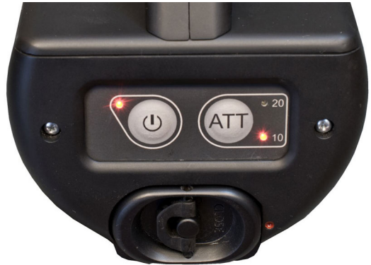
Fig. 11 Detector is switched-on with -10 dB input signal attenuation
