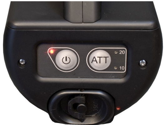
Fig. 12 Detector in a maximal sensitivity mode
